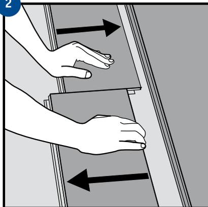
Disassemble the panels by sliding horizontally. (Do not fold up.)
